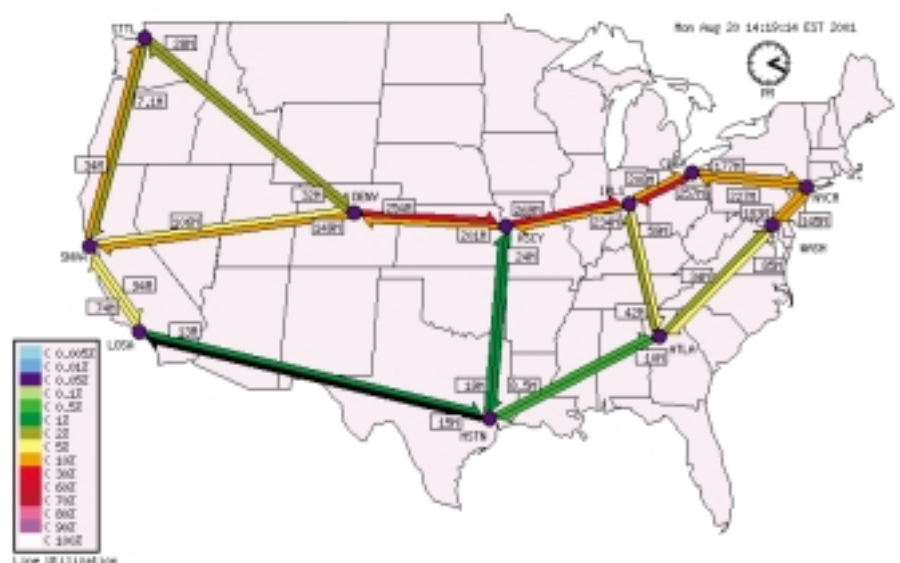
Figure 2: 'Weather map' of the traffic load on the core links of the Abilene network. (Courtesy of the Abilene Network Operations Center, Indiana University, http://hydra.uits.iu.edu/~abilene/traffic/ )
